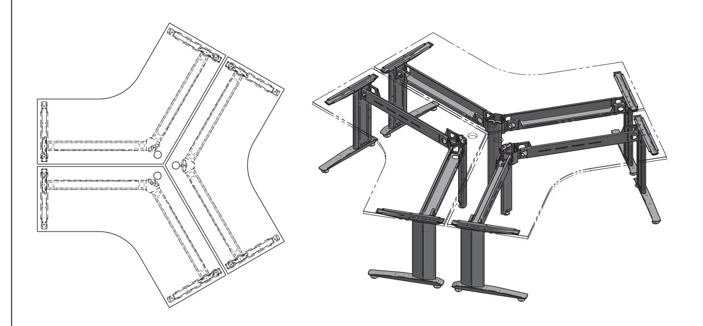
Height 720mm Back edge length 1200 – 1350mm Depth 700 – 800mm
